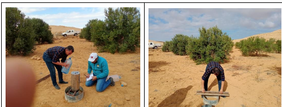
Figure 27. Field photo during the experiment of infiltration test at Wadi El Agarma
